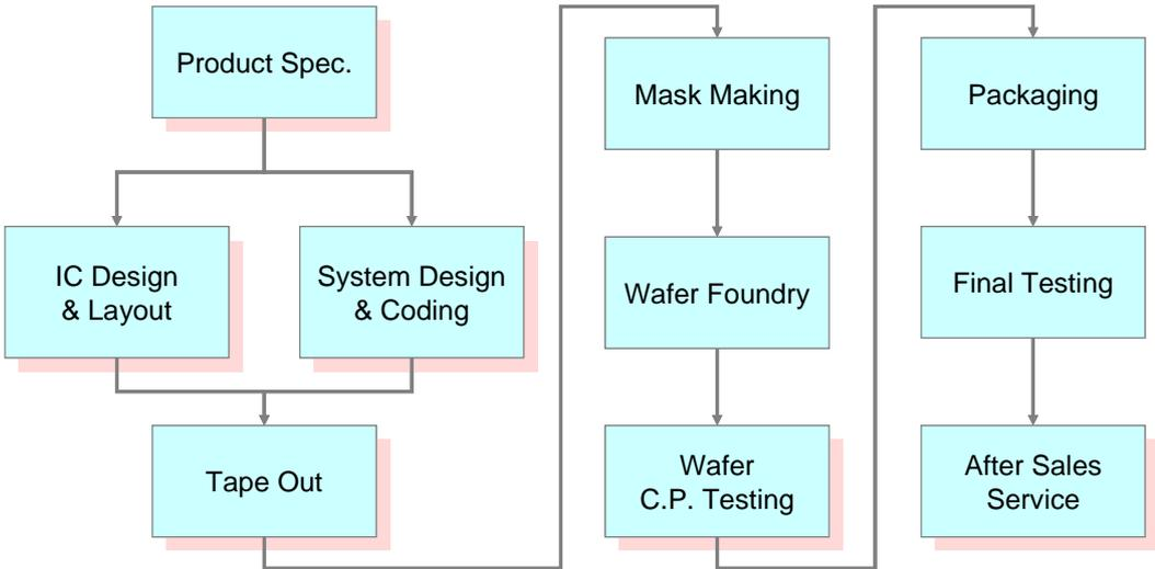
In the product development flow, Sunplus focuses on IC design, system design, wafer testing and sales services but out-sources most aspects of the manufacturing including mask making, wafer fabrication, packaging, and final testing.
