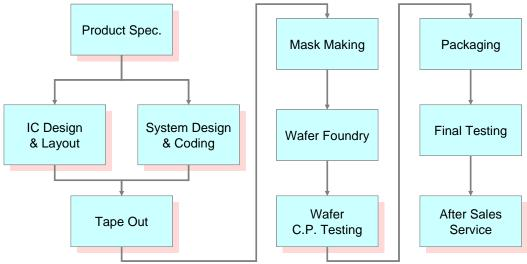
In the product development flow, Sunplus focuses on IC design, system design, wafer testing and sales services but out-sources most aspects of the manufacturing including mask making, wafer fabrication, wafer sawing, packaging, and final testing.
